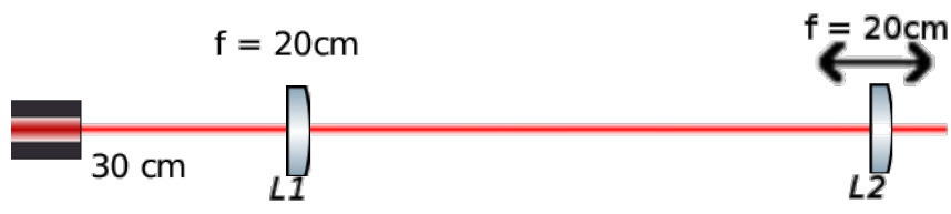
Figure 17: The setup of an optimization usage of theia , the position of L2 is varied in order for the waist of the final beam to be as large as possible.
